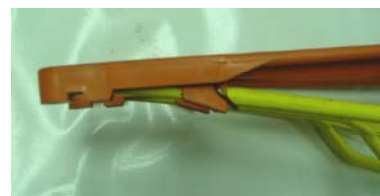
Hog Ring Installed on 3- point guard
