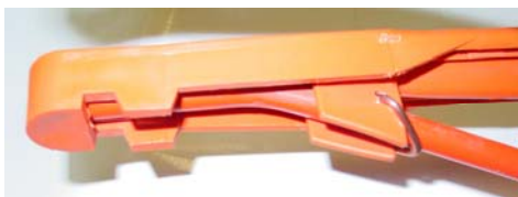
Hog Ring Installed on 6- 7- or 8- point guard
